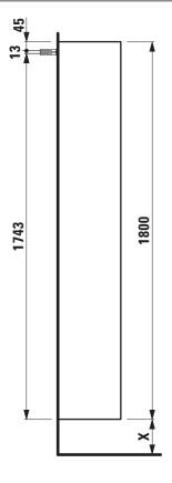
X = The exact hight must be set during installation.
